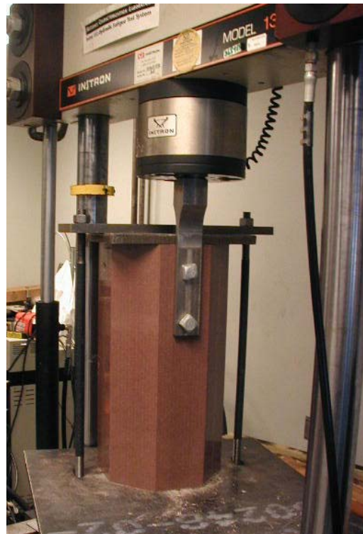
Test Setup for Bearing Hole Tests
