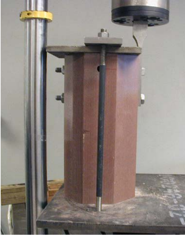
Test Setup for Bearing Hole Tests
